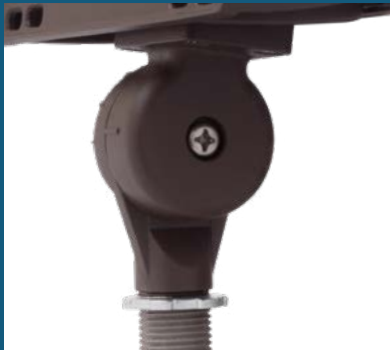
Adjustment range of 0° to ±90° & ½” threaded connector with locking nut
