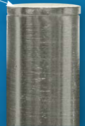
Close-up of Silver-Nickel Contact Tip
